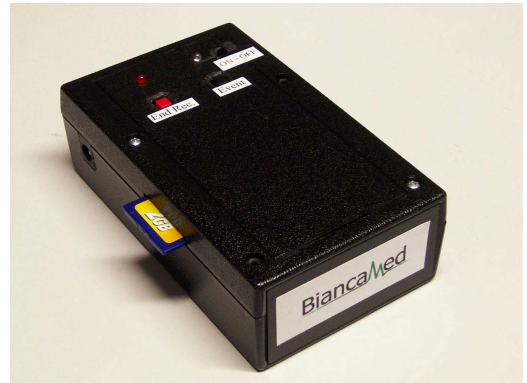
Fig. 1. Shown is the BiancaMed data logger unit. The dimensions are length 116mm, width 70mm, and height 36mm.
